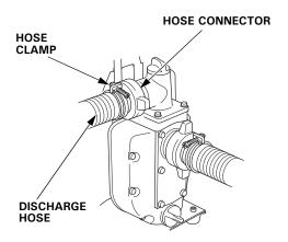
Tighten the hose clamp securely to prevent the discharge hose from disconnecting under high pressure.
