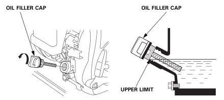
3. Reinstall the oil filler cap.
