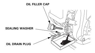
4. With the engine in a level position, fill with the recommended oil to the upper limit of the oil filler neck (see page 32).
