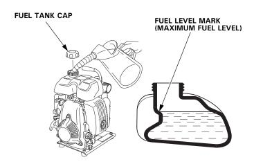
After refueling, reinstall the fuel tank cap securely.
