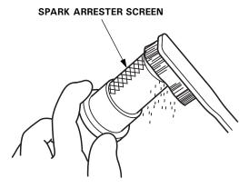
4. Install the spark arrester and the muffler protector in the reverse order of disassembly.
