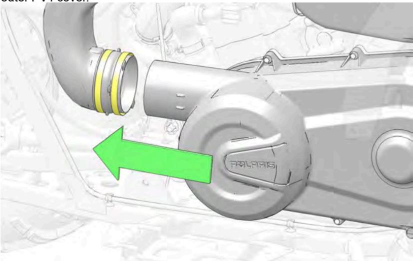
6. Loosen the PVT outlet duct clamps.
