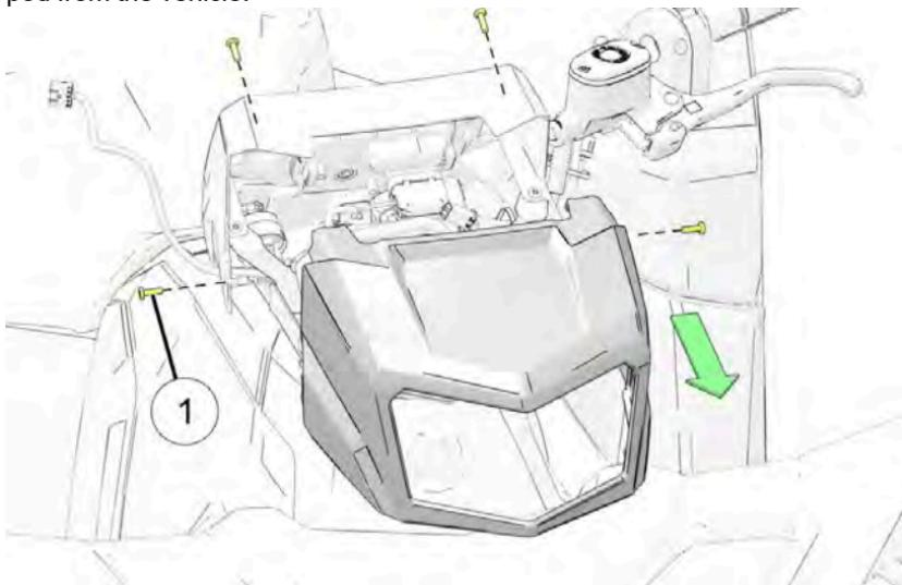
2. Disconnect the main wiring harness ② from the back of the headlight housing.
