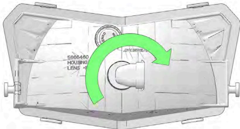
5. Connect the main wiring harness to the back of the headlight housing.
