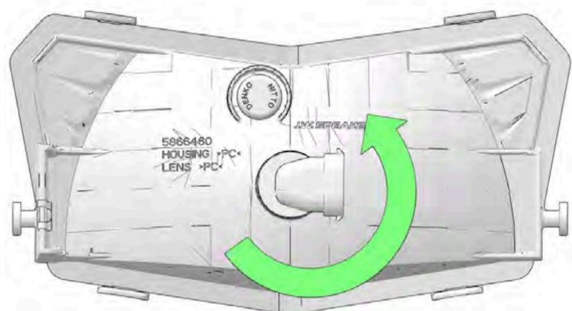
4. Apply dielectric grease to the socket and install a new lamp. Turn the lamp socket clockwise to secure the lamp into place.
