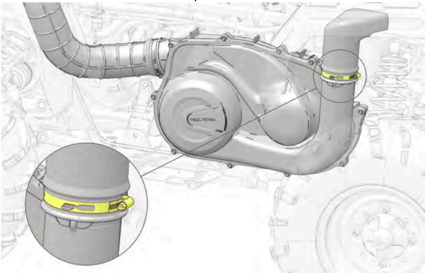
8. Torque the PVT outlet duct clamp to specification.
