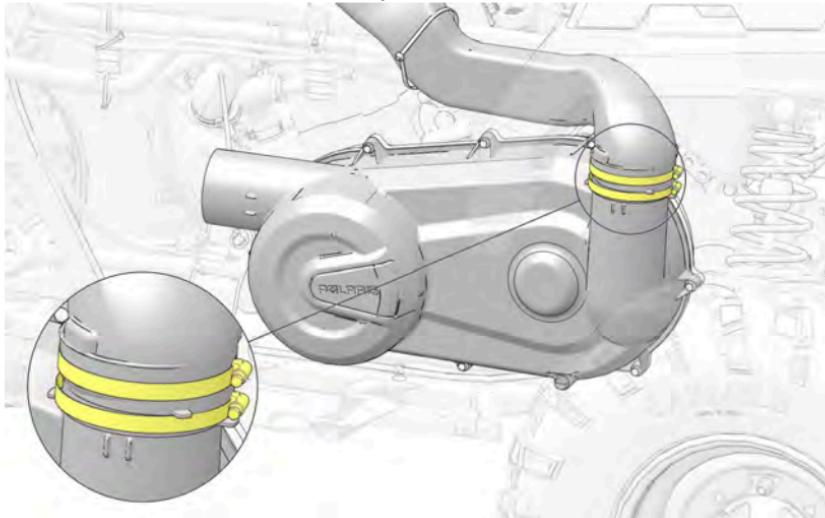
6. Install the PVT inlet duct and clamps.
