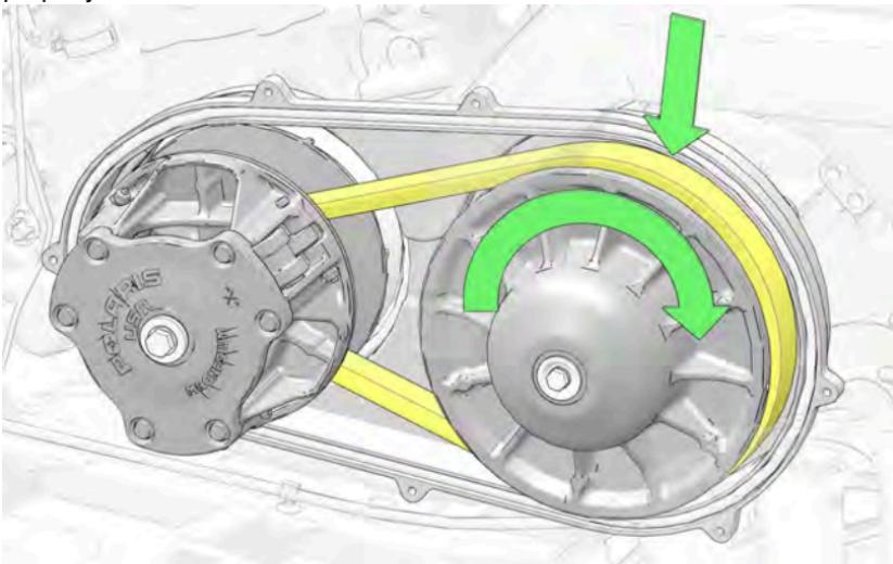
4. Install the outer PVT cover and 8 fasteners. Torque fasteners to specification.
