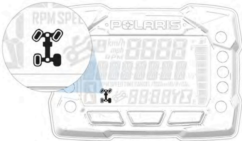
The All Wheel Drive (AWD) system is controlled by the Driveline Switch. Engage AWD before getting into conditions where AWD may be needed. If the rear wheels are spinning, release the throttle before switching to AWD.
