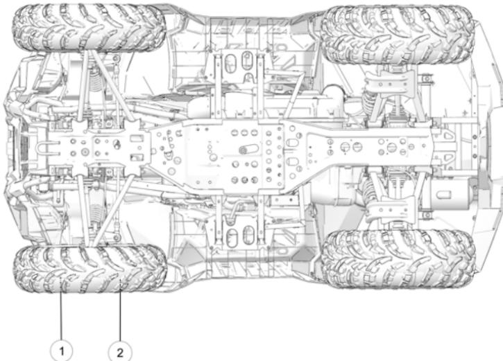
Use the following procedure to check the toe alignment of the vehicle. The recommended toe alignment is 1/4-1/2 inch (6-12 mm).
