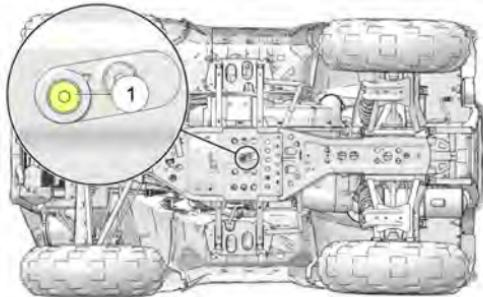
1. Position the vehicle on a level surface and put the transmission in PARK (P). Stop the engine and lock the temporary brake lock.
