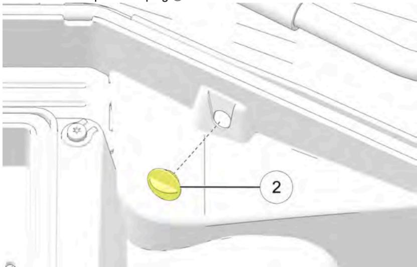
9. Insert the Torx® wrench tool ③ (included in your vehicle's tool kit) through the compartment plug hole to access the top center screw ④ on the back of the front bumper light. Loosen the screw.
