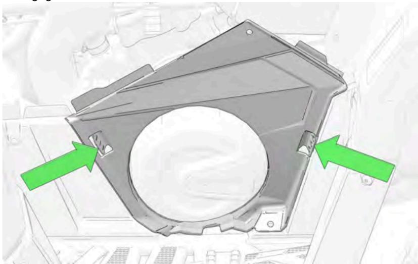
5. Remove the two screws and two push rivets from the footwell.
