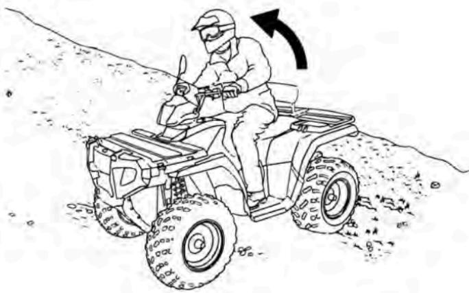
Driving on a sidehill is not recommended. Improper procedure could cause loss of control or overturn. Avoid crossing the side of any hill unless absolutely necessary.
