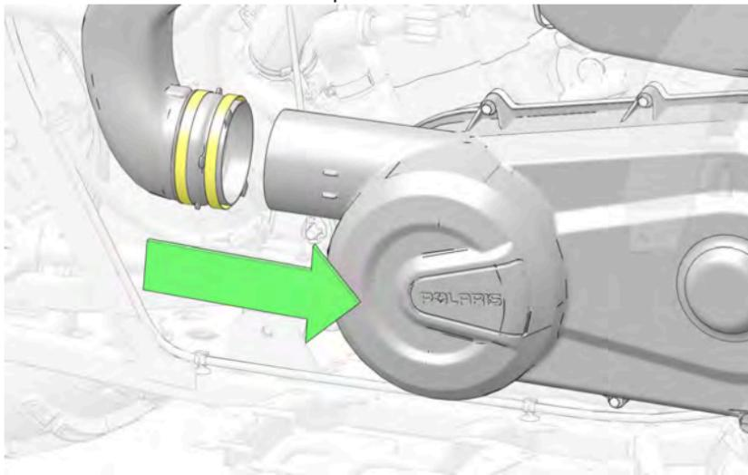
7. Torque the PVT inlet and outlet duct clamps to specification.
