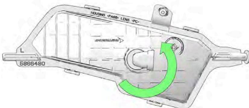
3. Apply dielectric grease to the socket and install a new lamp. Turn the lamp socket clockwise to secure the lamp into place.
