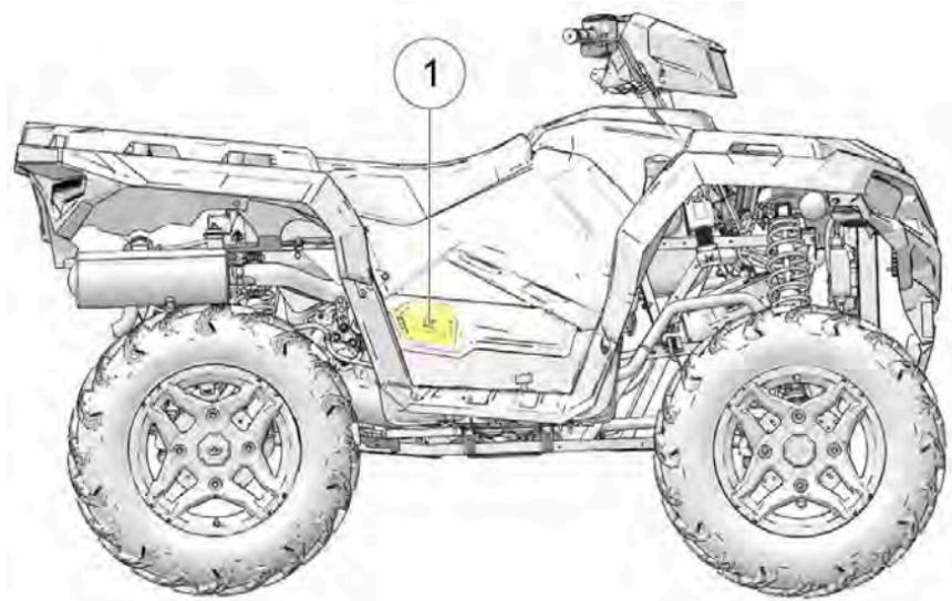
1. Position the vehicle on a level surface and put the transmission in PARK (P). Stop the engine and lock the temporary brake lock.
