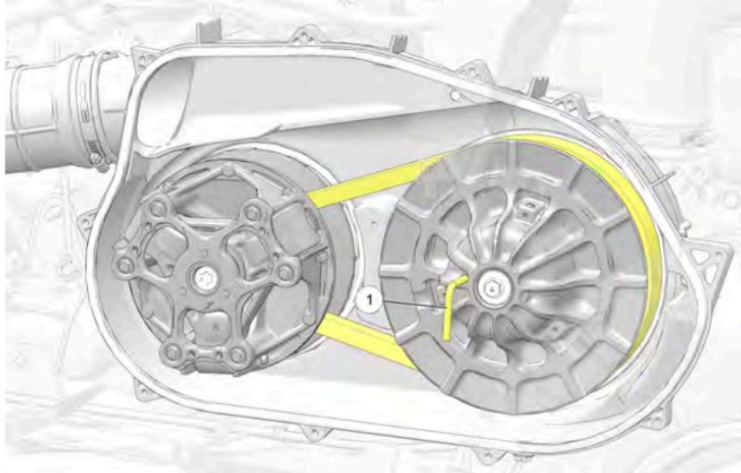
3. Rotate the driven clutch and walk the belt into the clutch.
