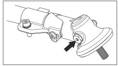
The grease in the bevel gear does not need to be changed unless repairs are carried out.
