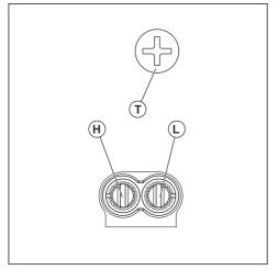
Turn the H-jet and L-jet clockwise to get less fuel in the mixture and counterclockwise to get more fuel in the mixture. Less fuel in the mixture gives a higher engine speed and more fuel in the mixture gives lower speed.
