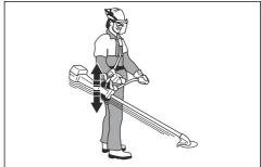
If the operation is to cut grass, let the cutting attachment stay lightly on the ground. Adjust the harness clamp to balance the product correctly.
