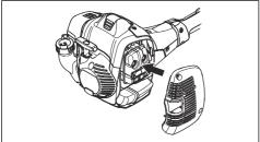
3. Remove the screw holding the spark arrestor mesh.
