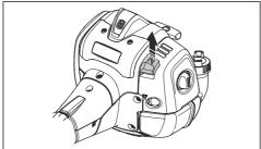
2. Remove the air filter cover and remove the air filter.
