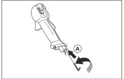
If the start throttle speed is too high, turn the adjuster screw (A) counterclockwise until the cutting attachment stops. Turn the adjuster screw (A) clockwise 1/2 turn more.
