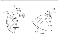
5. Remove the cutting attachment guard (A).
