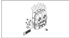
4. Clean the spark arrestor mesh if it is blocked or replace it if it is damaged.
