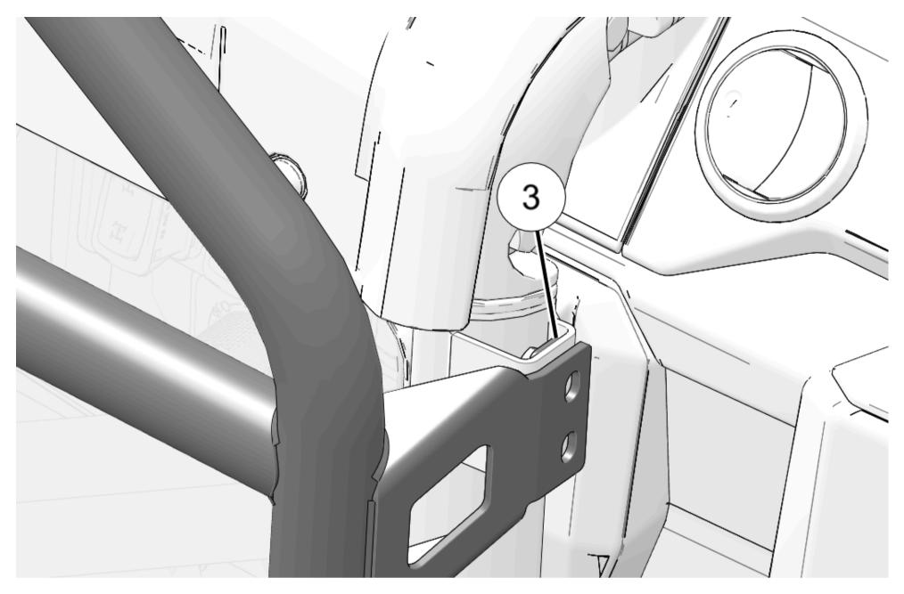
7. Put upper door hinge between headache rack mount and hinge mount.
