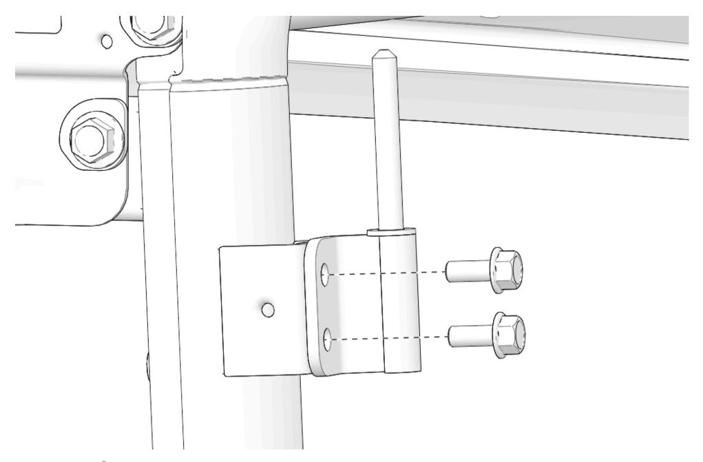
5. Put headache rack ② in position on vehicle. Line up mounts with hinge mounts on vehicle ROPS.
