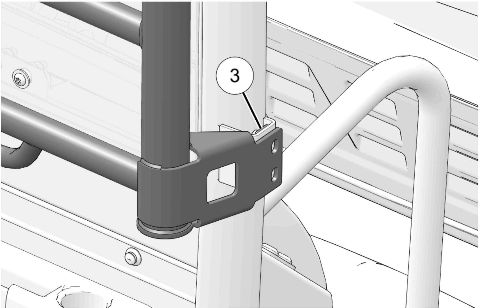
10. Install steel spacer ① between headache rack and hinge mount.
