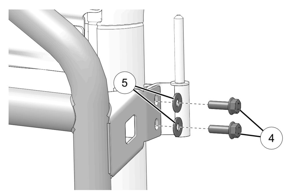
9. Install hinge plate 3 on inside of lower hinge mount.
