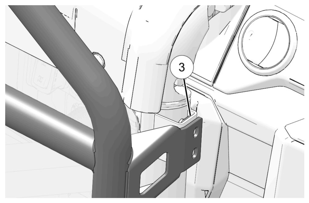
3. Put steel spacer (1) in between headache rack mount and hinge mount.
