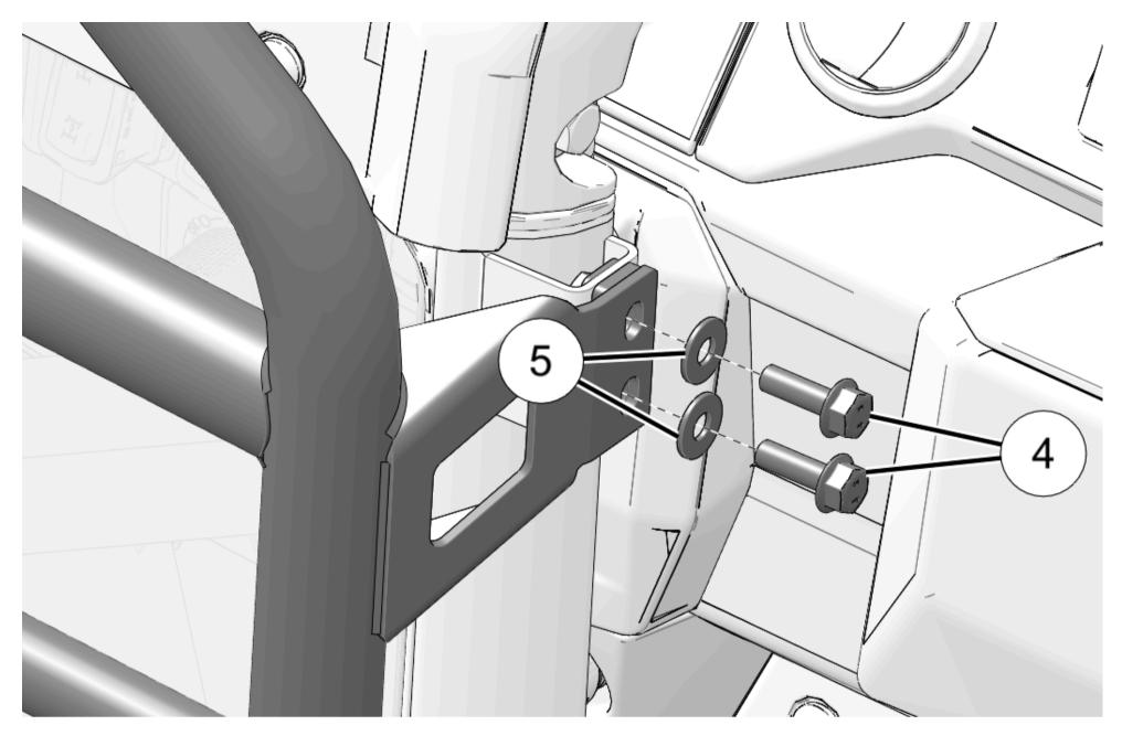
7. Put upper door hinge between lower headache rack mount and lower hinge mount. Make sure bushing is installed.
