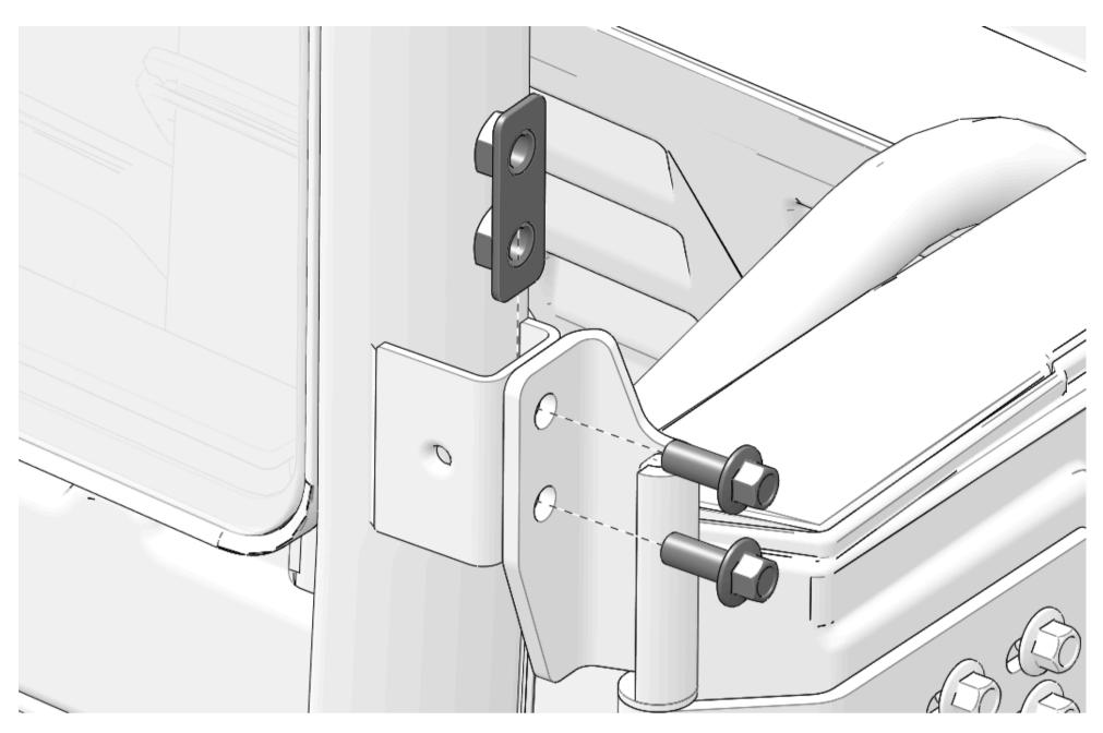
2. Remove and keep upper door hinge and hinge bushing.
