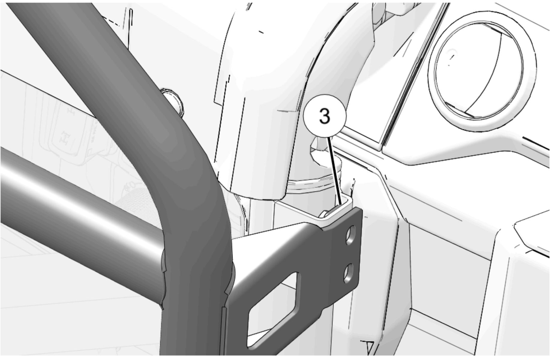
7. Put upper door hinge between headache rack mount and hinge mount.
