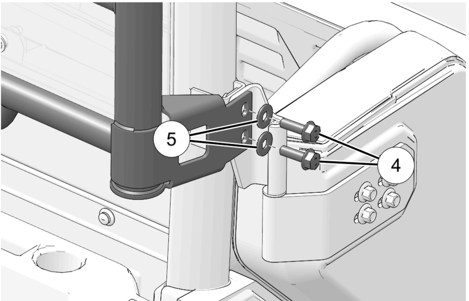
9. Torque all screws ④ to specification.
