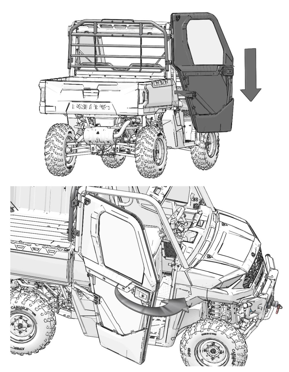
13. Install nut on lower door hinge. Tighten until snug. Make sure door turns without binding or free play.
