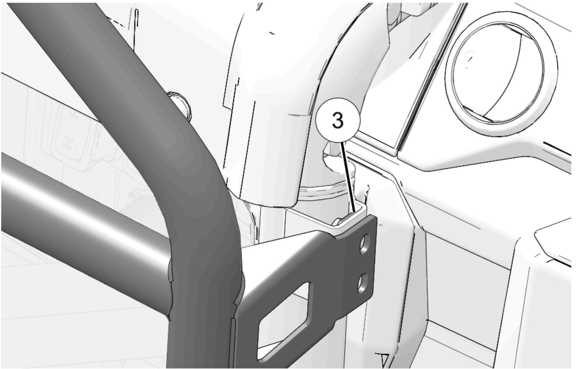
3. Put steel spacer ① in between headache rack mount and hinge mount.
