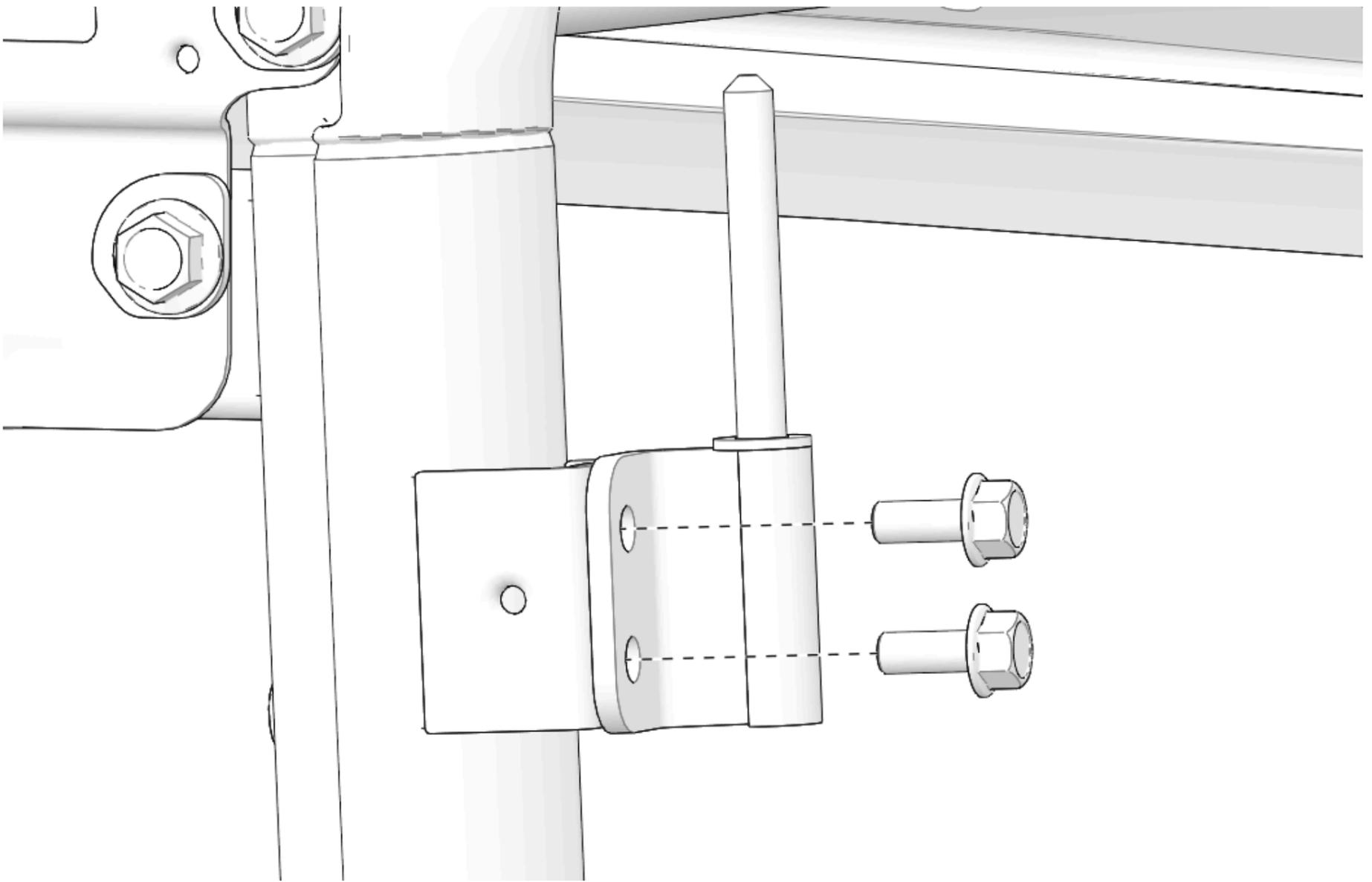
5. Put headache rack ② in position on vehicle. Line up mounts with hinge mounts on vehicle ROPS.
