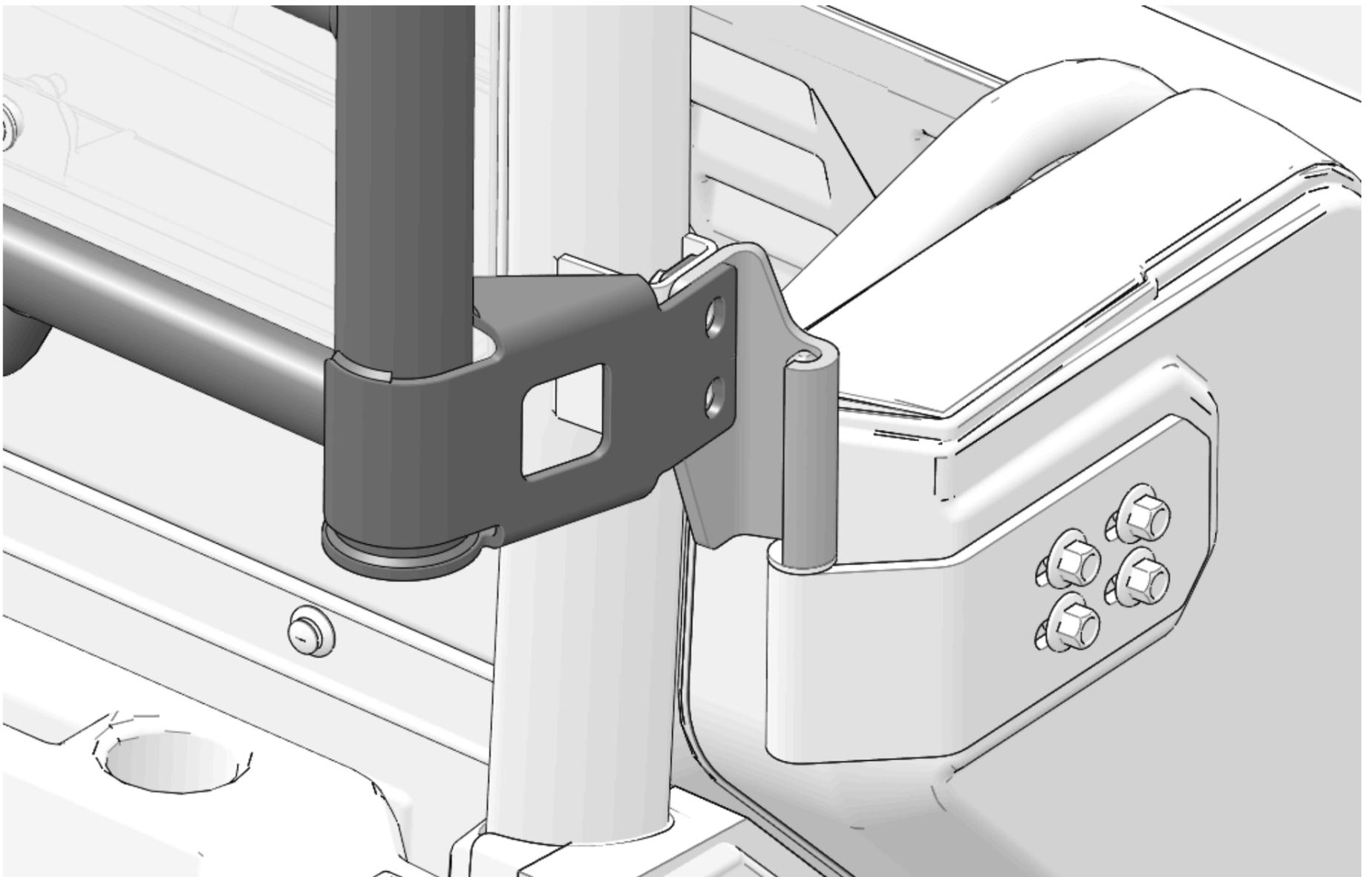
8. Loosely install two washers ⑤ and two screws ④.
