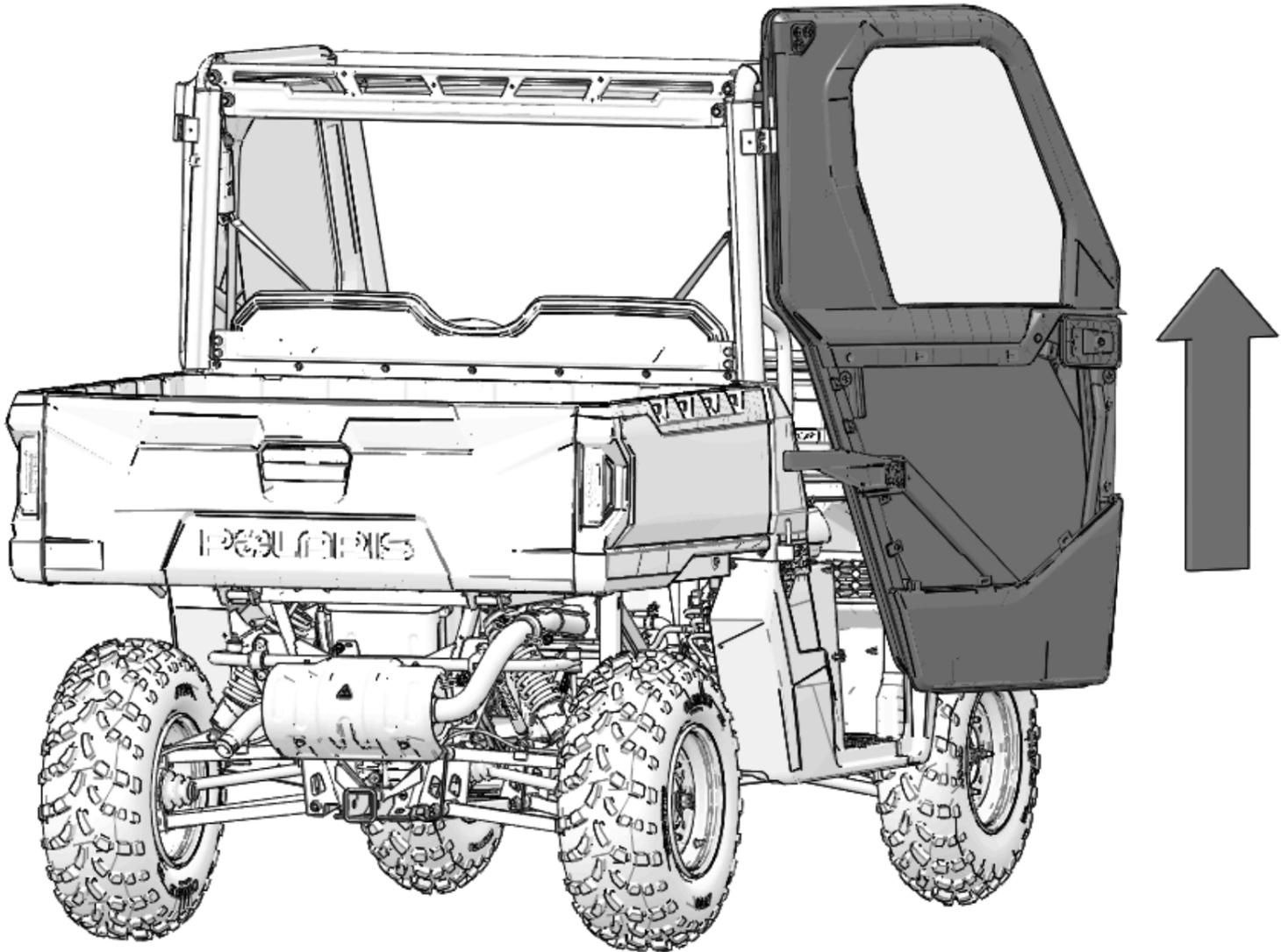
4. Remove upper door hinge and hinge bushing.
