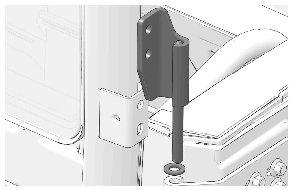
3. Put headache rack (2) in position on vehicle. Line up mounts with hinge mounts on vehicle ROPS.
