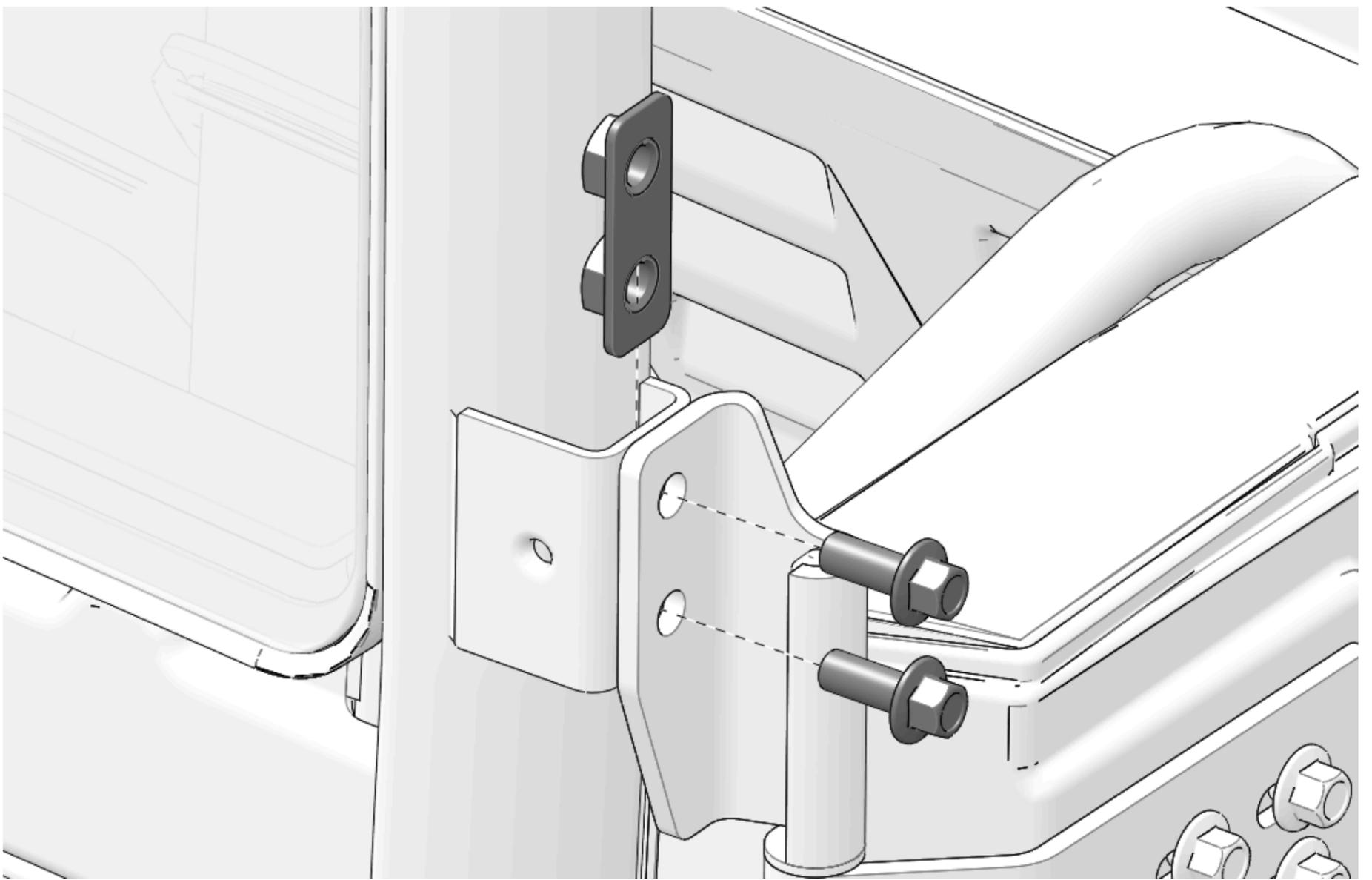
2. Remove and keep upper door hinge and hinge bushing.
