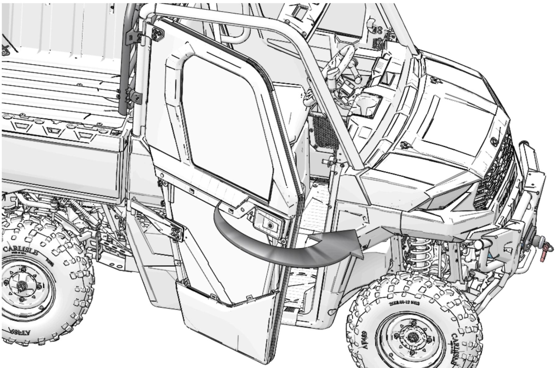
13. Install nut on lower door hinge. Tighten until snug. Make sure door turns without binding or free play.
