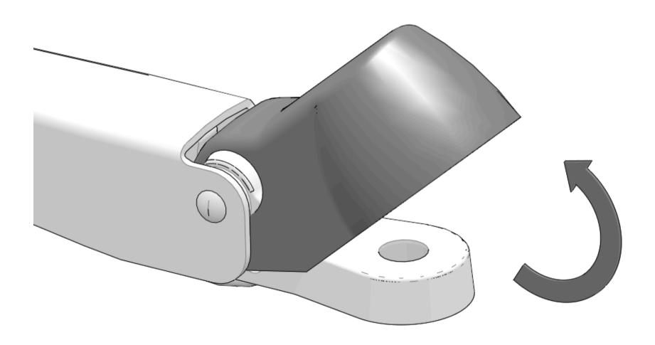
12. Put wiper arm on to wiper arm shaft in a position that will allow wiper blade to fully clean windshield.
