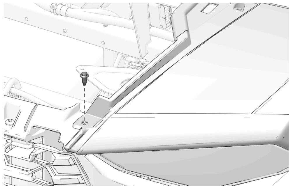
33. Install rear of left hood with one kept screw.
