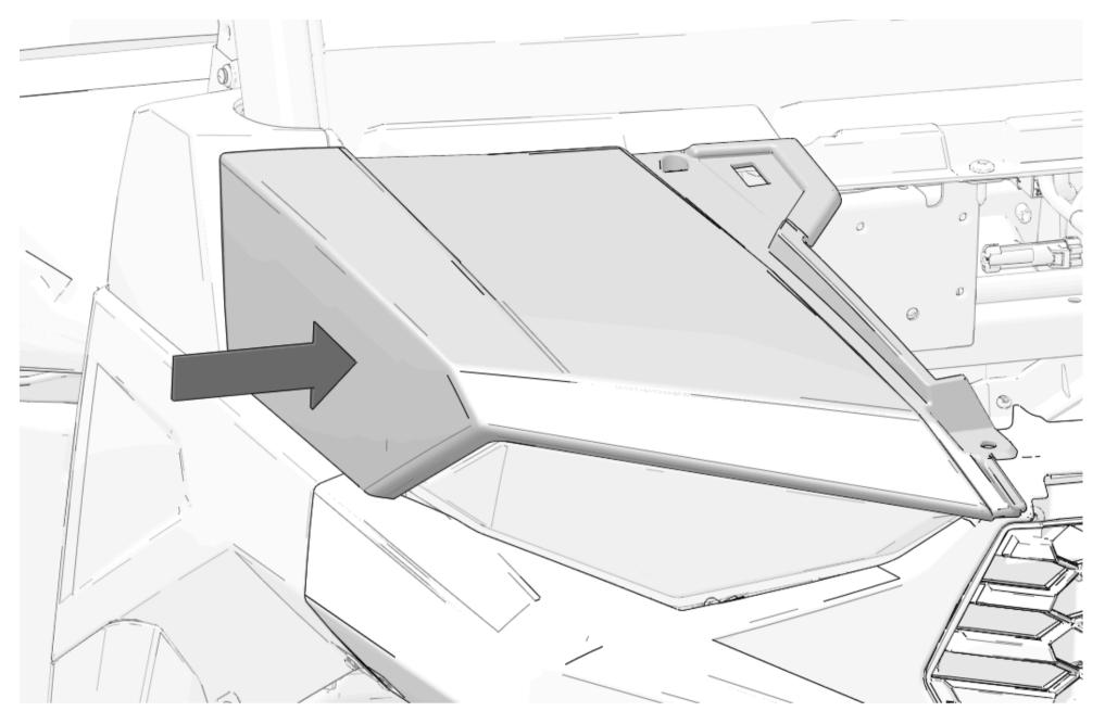
2. Install front of right hood with one push-pin rivet.
