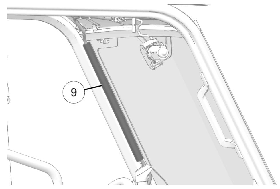
25. Route wiper harness 29 up along ROPS and through routing channel 9 toward wiper motor 6.
