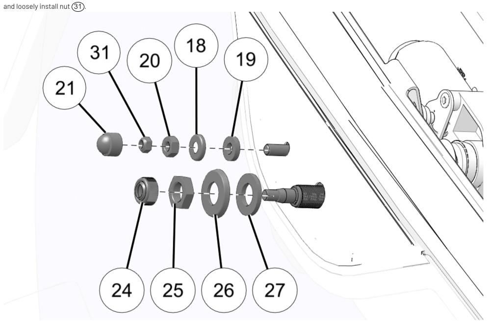
8. Install washer 27, washer 26 and loosely install nut 25
