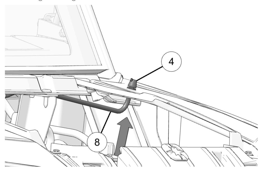
35. Torque left hood screw to specification.
