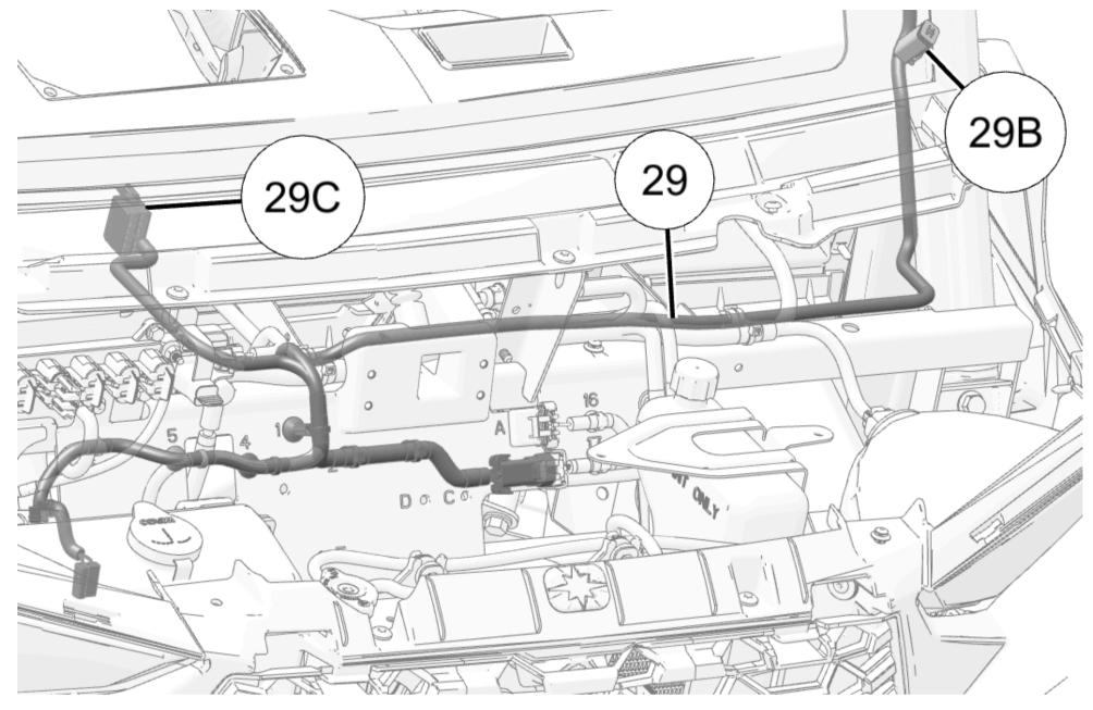
15. Route connector **29A** on wiper harness **29** to connector **30A** on wiper fuse harness **30**.
