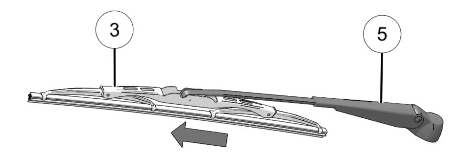
11. Lift wiper arm cap to reveal mounting bracket.
