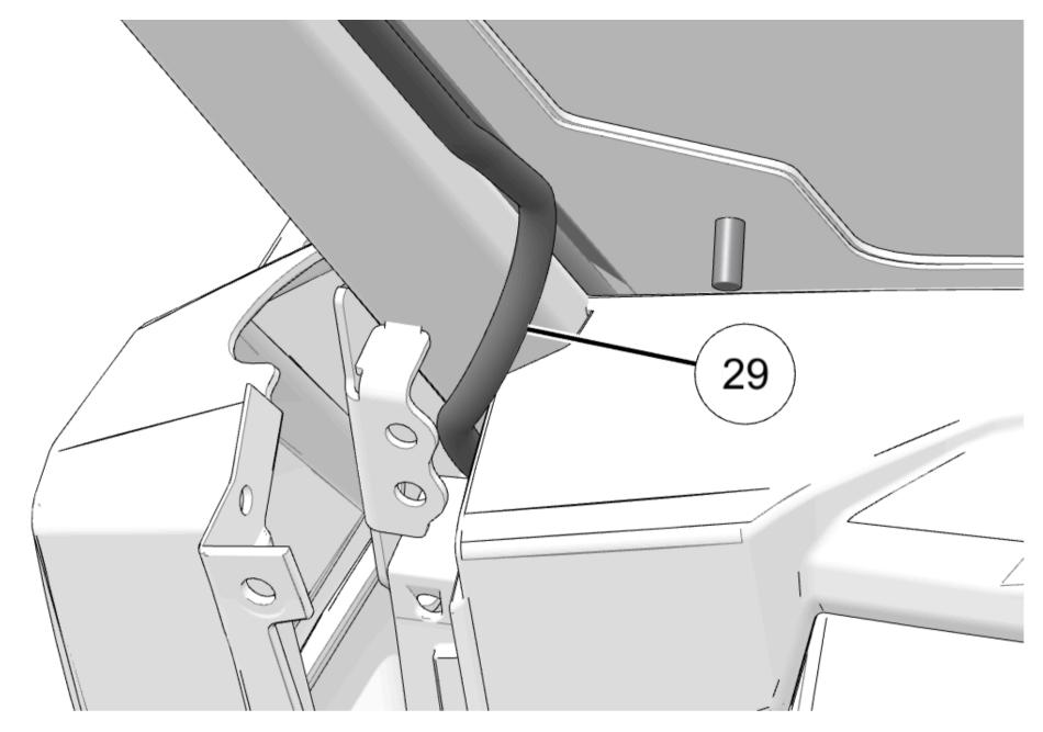
$23. \ In stall \ three \ kept \ fasteners \ to \ front \ left \ fender \ flare.$
