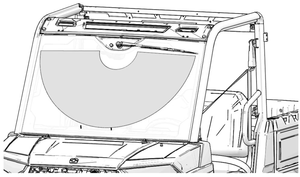
13. Install wiper with washer 23 and nut 22.
