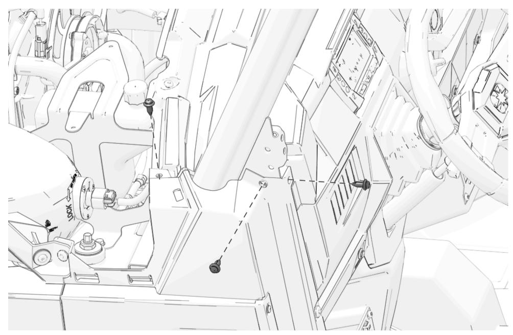
24. Remove and discard backing from routing channel (9) and install on ROPS.
