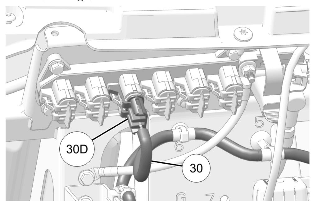
18. Install fuse **30B** and **30C** on wiper fuse harness 30 to under hood panel.
