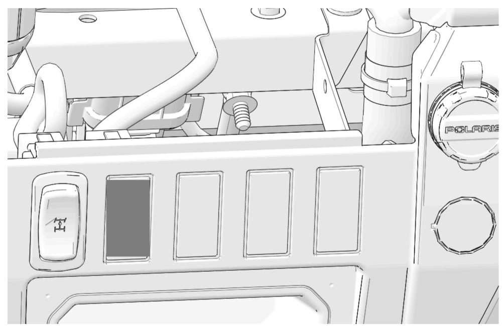
20. Install switch (7) to switch connector **29C** on wiper harness (29). Push switch (7) into control panel until switch tabs click into place.
