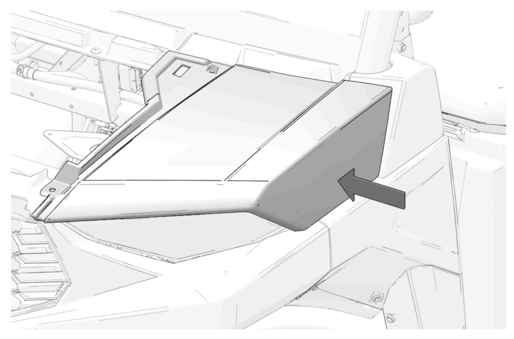
$\ensuremath{\mathtt{32}}.$  Install front of left hood with one push-pin rivet.
