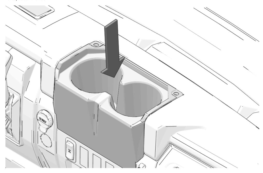
2. Install cup holder with two kept push-pin rivets.
