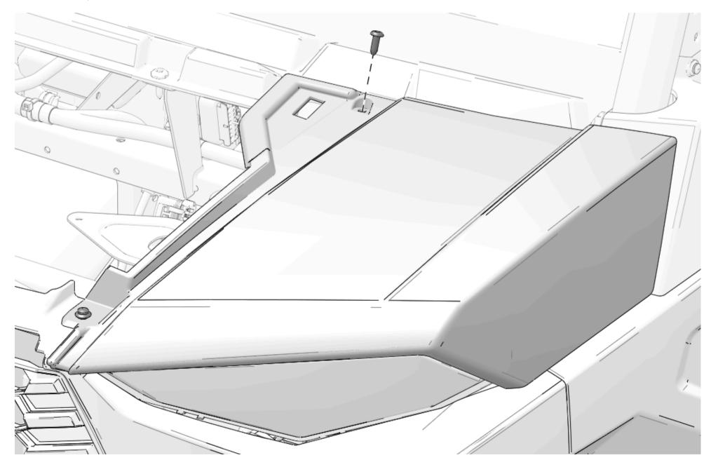
2. Remove and keep one push-pin rivet from outer hood.
