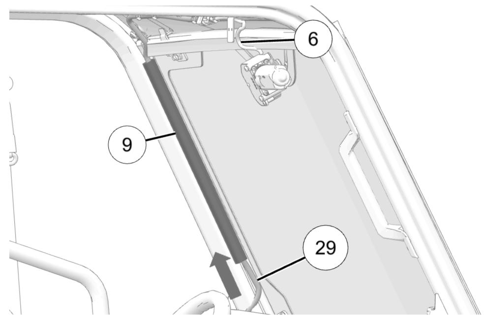
26. Attach wiper harness 29 to ROPS with installed edge clips and connect **29B** to wiper motor 6.
