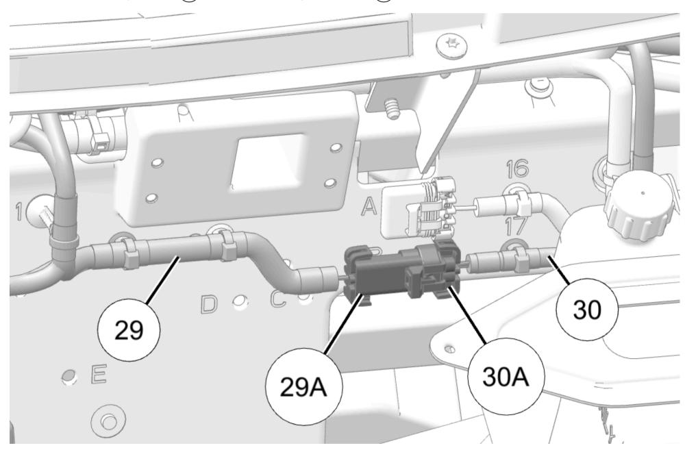
16. Connect **29D** on wiper harness **29** to washer pump **1**.
