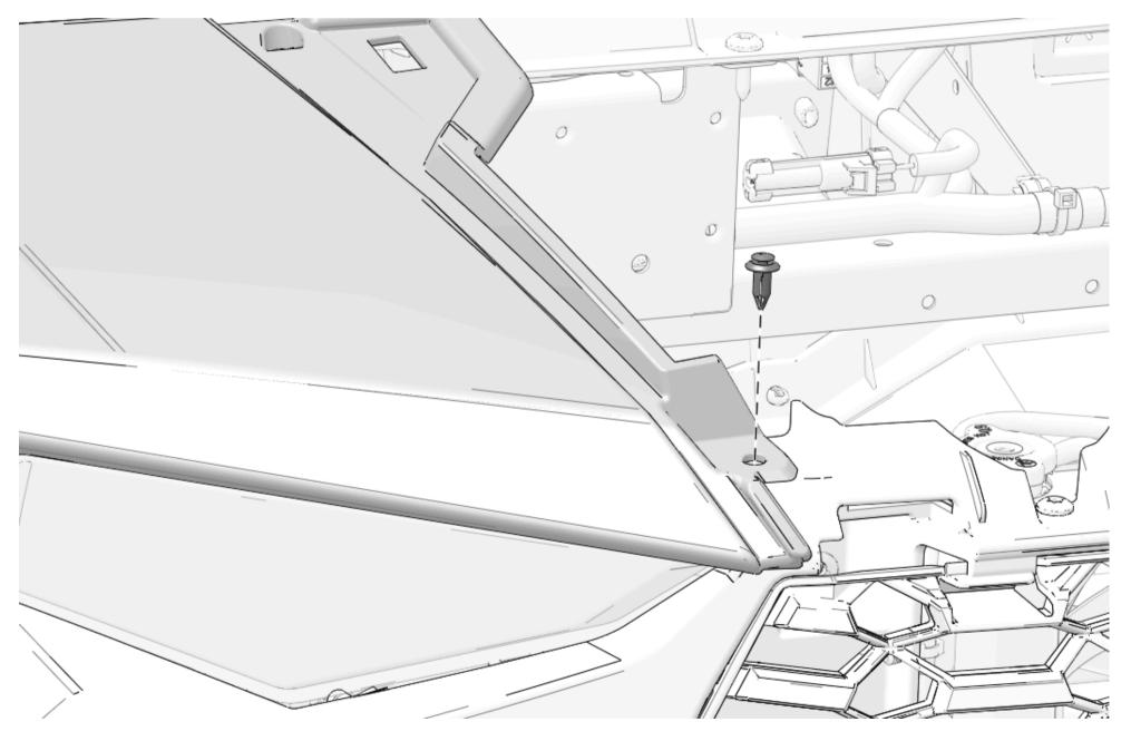
$\ensuremath{\mathtt{3}}.$  Install rear of left hood with one kept screw. Torque to specification.
