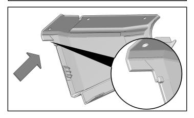
8. Align the side bezel retention tabs with the body of the vehicle, pressing the bezel into place until fully seated. Continue by reinstalling the three push-pin rivets into the side bezel.
