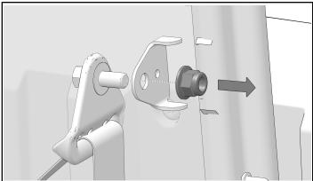
27. Insert the fastener through the seat belt mounting point, washer and the limiter strap post mount (1) with the tab up and facing inward. Continue by inserting the assembly into the ROPS bracket and reinstall the nut. Torque the nut to specification.
