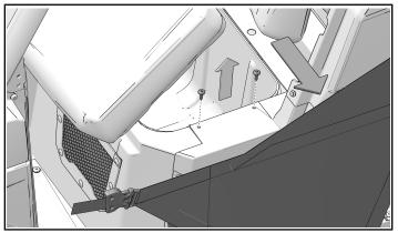
8. Reinstall the retained fasteners and torque to specifications. Lift up the two seat belt buckles and pivot the seat back down.
