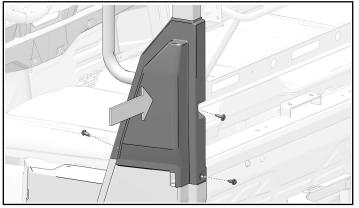
9. Reinstall the retained fastener and clamp over the grab handle into the side bezel and torque the fastener to specification.
