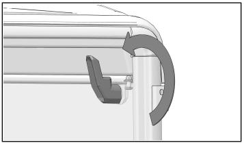
10. Continue by pivoting the rear panel in and locking the panel, if installed.
