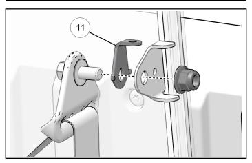
28. Next, install a fastener (1) and spacer (7) into the top of the limiter strap post mount (1) and secure with a nut (18). Align the hole in the limiter strap with the limiter strap post and press the strap down around the post. Continue by torquing the fastener to specification.
