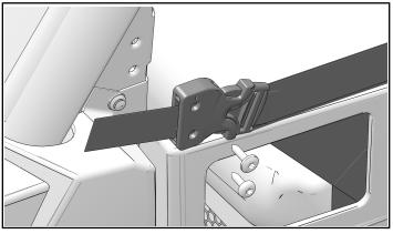
3. Remove and retain the lower side net fastener on the floorboard. Continue by reinstalling the retained lower fastener and torquing to specification.
