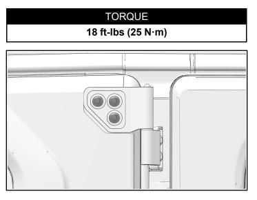
21. Torque the lower door hinge fasteners to specification.
