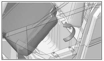
7. Remove and retain the two side net fasteners and set net aside.
