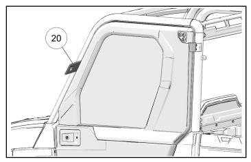
20. Torque the upper door hinge fasteners to specification.
