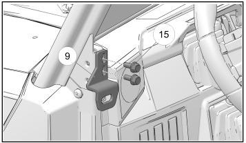
17. Loosely install the striker (6) and round washer (19), round side out, into the striker mount (9) and ecure with a nut (17).
