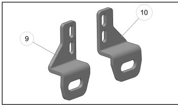
16. Loosely align the striker mount (9) with the mounting holes on the ROPS and install two new fasteners (5).
