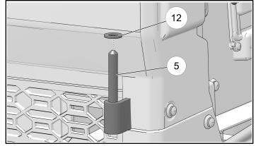
12. With the aid of an assistant, align the upper and lower door hinges with the chassis hinges while door is in the open position. Pivot the door as needed to fully seat the upper and lower hinges.
