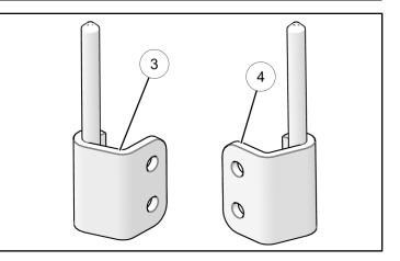
Align the upper chassis-hinge with the mounting holes on the ROPS bracket. Install two fasteners
