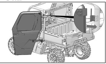
13. Press shim door adjustment tool (13) onto the lower door frame.
