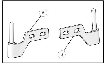
6. Align the lower chassis-hinge (5) with the mounting holes on the rear of the cab and install two fasteners. Align the bracket in the middle of the adjustment range and torque the fasteners (15) to specification while ensuring the bracket remains level.
