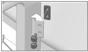
2. Remove the fasteners from the side net latch on the ROPS and remove the latch.
