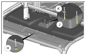
iii. Carefully pull LH and RH edges of liner from between ROPS and roof seal. Set liner aside.
