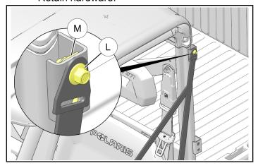
b. Install light assembly ① (with holder ②) and net anchor to upper ROPs mounting bracket using retained screw ①, new screw ③, and retained nut plate ๋.
