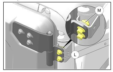
b. Install light assembly ① (with holder ②) to upper ROPs mounting bracket using retained screws ① and nut plate ⑩. Align holder with lower ROPS mounting bracket, then tighten screws.
