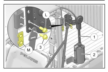
c. Install holder ② to lower ROPs mounting bracket using two screws ③ and nut plate ④. Tighten screws.
