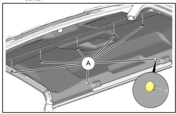
c. Remove two each screws ® and washers © (if installed).
