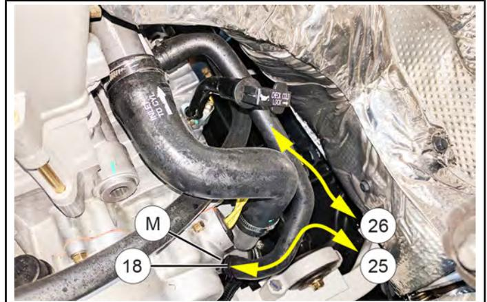
6. Install **HOT SUPPLY** heater hose between 3-way valve and engine
